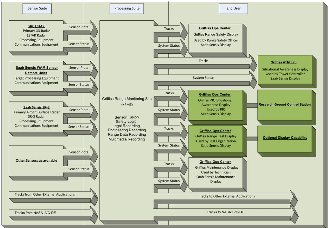
**Figure 4 Griffiss WAM-Based Instrumentation System Architecture**
